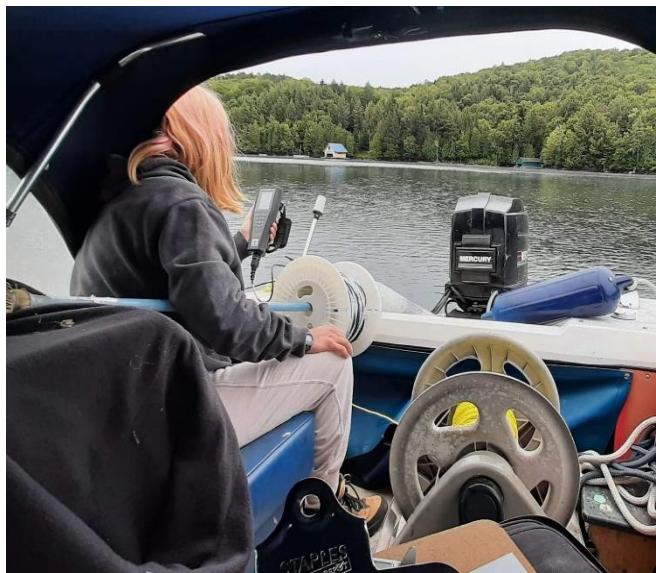
**Photo 1:** Environmental technologist taking the dissolved oxygen and temperature profile of Bark Lake, using a DO and temp probe.
