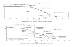
A landslide risk zone is the area inside a strip of land situated on both sides of the ridge line of an embankment. The strip of land that may be associated with a landslide risk zone is composed of three (3) distinct parts:
